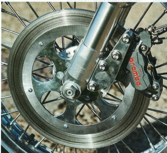
Up front, a Brembo racing four-piston caliper bites on a Barnes replica disc featuring a disc support machined in 7075 alloy in the Atelier Chatokhine workshops
