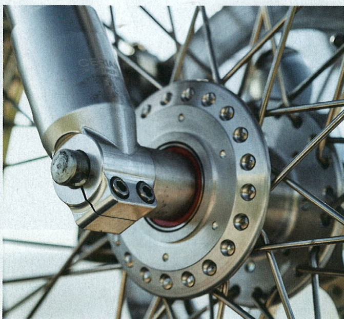
Front suspension is dealt with by fully adjustable, CR-Suspension GP38 forks – 38mm Ceriani replicas, with a quick-change Barnes-type alloy hub nestled at the bottom
