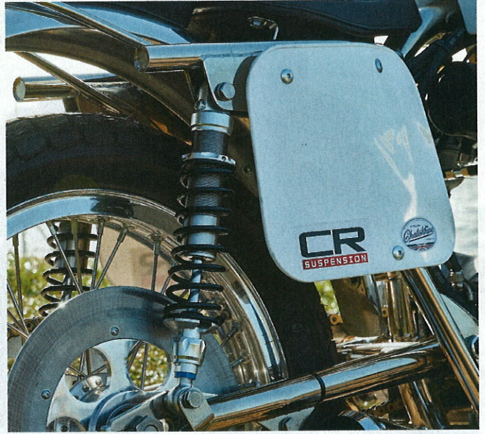
Frank Chatokhine swears by these CR-Suspension GS03AR CNC forged racing shocks, fully-adjustable for preload and rebound damping and with a CR-MO shock shaft
