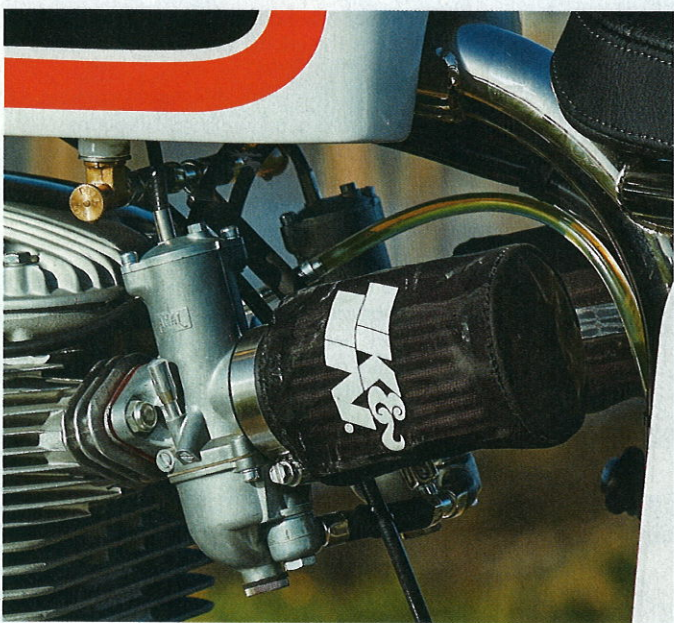
Fuelling is by a pair of 32mm Amal Mkl Premier Concentric 900s, with the spark to fire it provided by a Pazon Sure-fire electronic ignition system
