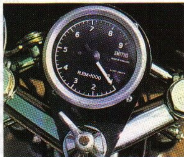
Smiths magnetic rev counter is fitted
