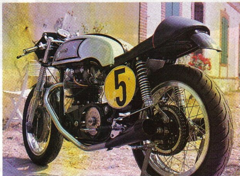
Hagons are used at the back of the Domiracer and Triumph conical hub
