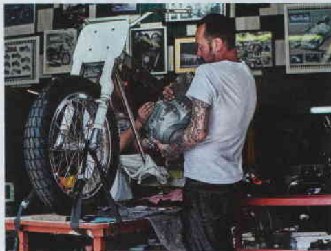
Bored-out A65 twin motor is wrestled into its new home
